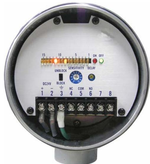
Secondly, systems based on the older diode detection technology have to have multiple sensitivity set points for any given detection range and are therefore not easy to set up requiring a complex three stage procedure to ensure satisfactory operation. By comparison the MicroSense is calibrated in one easy step via the sensitivity dial. The 15 LED indicator array at the
